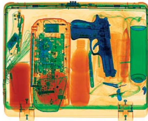
Color image: Materials are represented as orange for organic, blue for metal, green for inorganic (other than metal)
